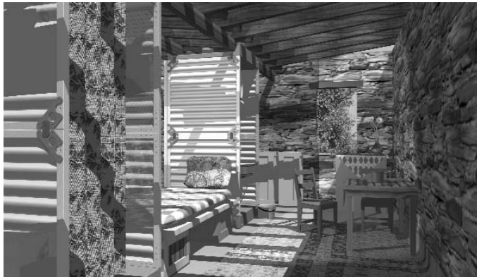
Interior Perspective of a unit inserted into house ruins where it acts as service core, structural support and scaffold for the construction of a larger dwelling.
